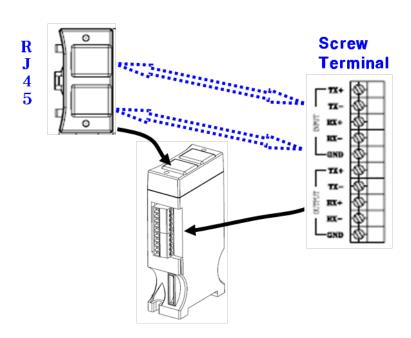
Serial connection through terminal/RJ45 for test of each module
