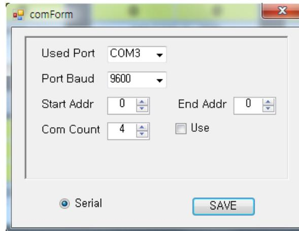
\*Com Count : This number is how many times of the error the user allows while the communication between PC and slave is executed. So if the communication error over allowed number is occurred, the followed such message with the address of errored unit is shown in the right bottom.
