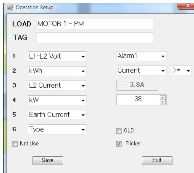
\*The kind of alarm factor is over/under current,unbalance current,earth current,power[KW],power factor(cos phi)h unit in system
