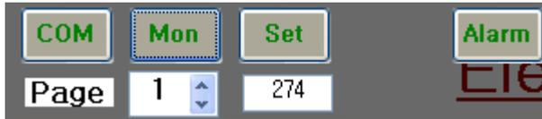
Alarm is shown as pressing F2 key, then the “alarm1” file in the folder in C>samdsbdb>DATA is created naturally.
