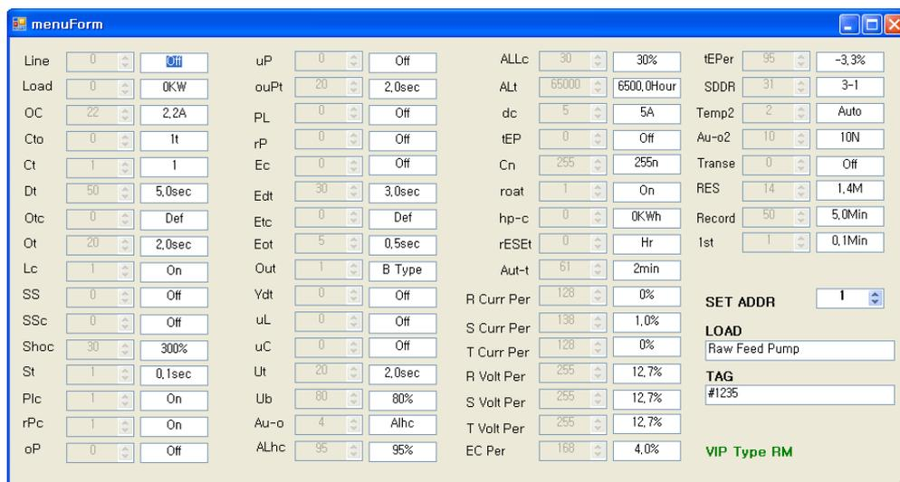
\*Reversely, the operator is able to change existed preset value or new preset value as activating another monitoring software “samdsp” ,but some of value according to product type is not matched completely with this “samdsp”
